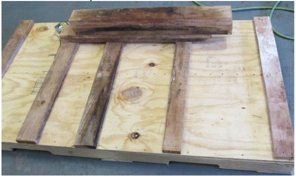
Set unit on pallet and secure with lag bolts
