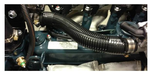
Torque all hose clamps to 31 in-lbs., and mark with a black paint marker as before
