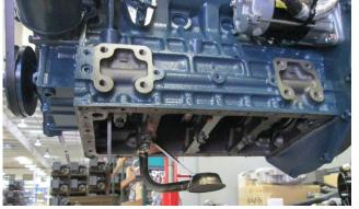
Insert the lubricated O-ring on the new sump, 16616-32115 and install on engine
