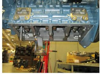
Remove the sump, and KEEP the O-ring on the old sump. Discard the removed sump
