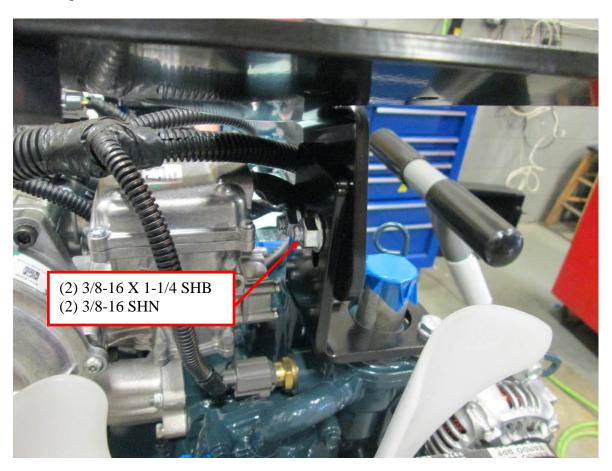
Install isolators on the top radiator mount
