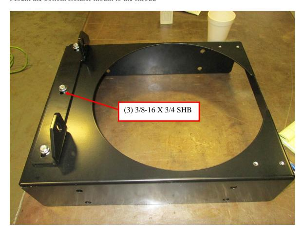
Install radiator shroud to the mounts
