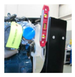
Center shroud about the fan and tighten all bolts
