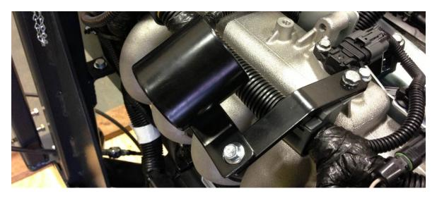
Install the cobra elbow on the air inlet on the engine
