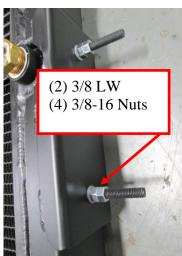
Apply Loctite 243 to the threads of the shoulder bolts
