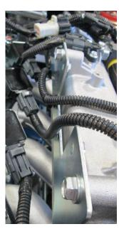
Install the removed isolators on the angled brackets
