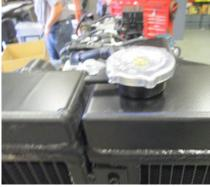
Install fittings into ports on the radiator/cooler
