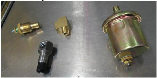
Remove existing oil switch and reinstall
