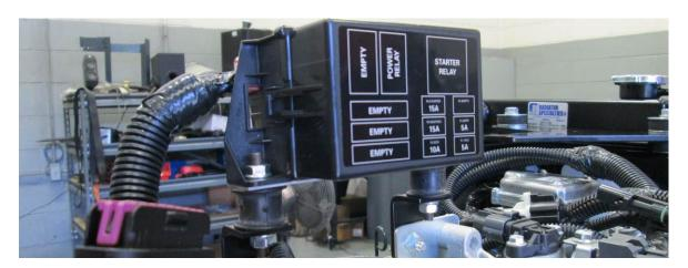
Add a piece of 5/8" loom, 6" long and tape up where the wires enter the fuse box
