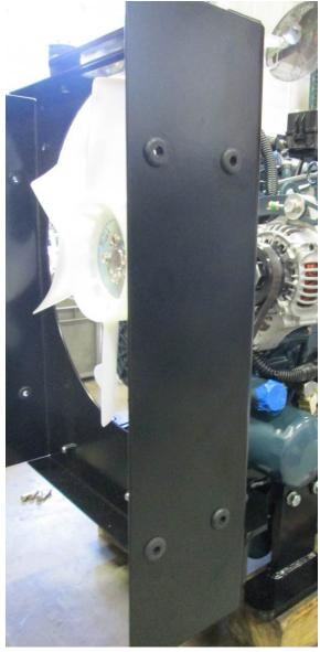
Assemble fittings into the radiator/cooler. Use Loctite 567 PST on all pipe threads
