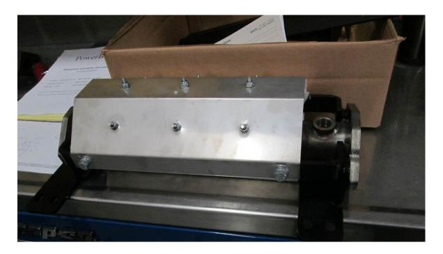
Place Cat in support brackets and install heat shield mounts
