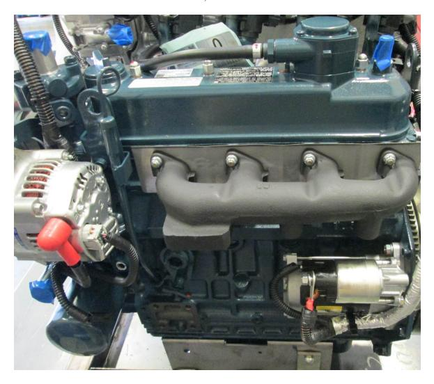
Reinstall manifold gasket and torque nuts to 13 Ft-lbs
