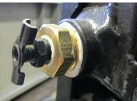
Install a low profile plug on the original port of the drain cock, and radiator cap
