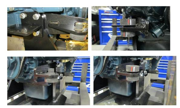
Mount the bottom isolator mount to the shroud
