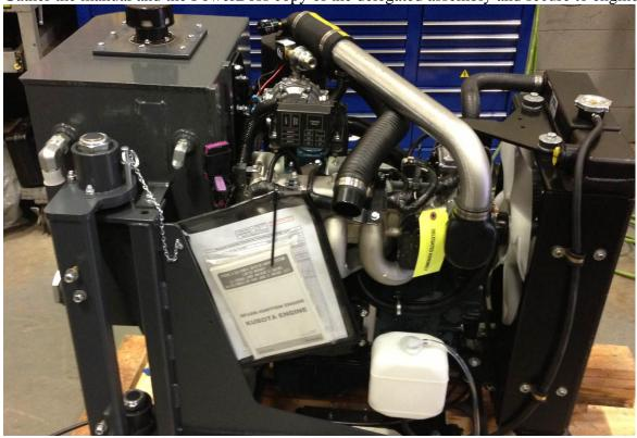
Have an inspector check over the unit and install the QC sticker near the serial tag
