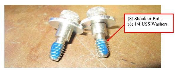
Install radiator into shroud **DO NOT USE AIR OR IMPACT TOOLS TO TIGHTEN SHOULDER BOLTS**
